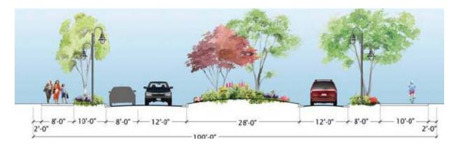
Within this 100 foot ROW, 32 feet is dedicated to the roadway—there are two 12 foot travel lanes and an 8 foot wide parking lane. There are separate pedestrian and biking trails, which, along with the associated greenspace, comprise 68 feet of the corridor.
