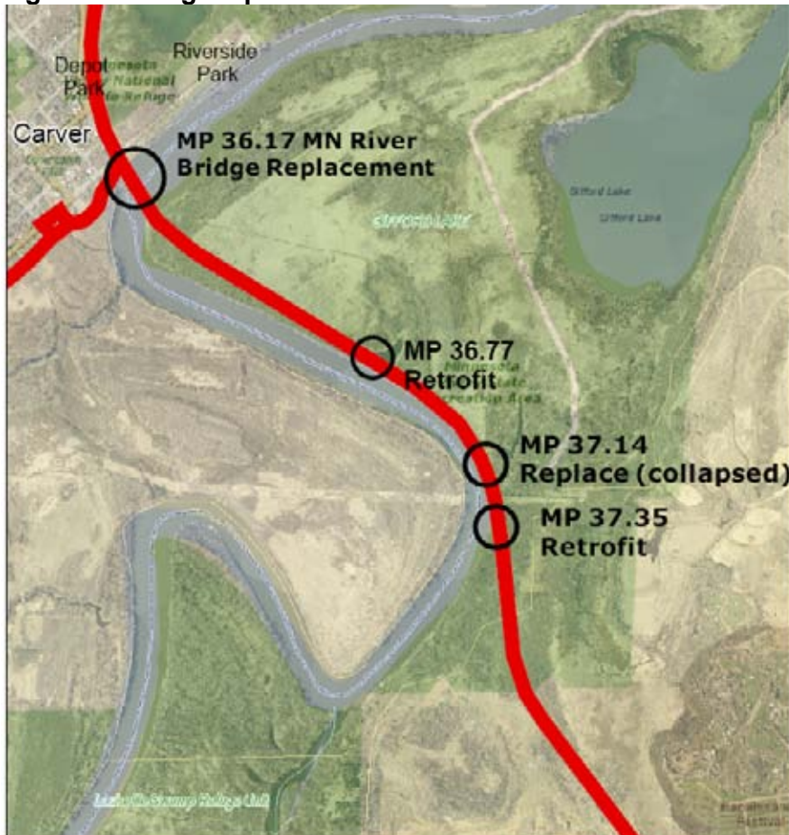
Figure 2: Bridge replacement or retrofit locations
