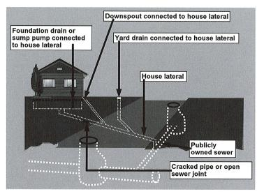
Inflow occurs in direct proportion to rainfall. The typical source is water from rain leaders, basement sump pumps (designed to capture water that enters basements) or foundation drains illegally connected directly to a sanitary sewer pipe. A sump pump can contribute 7,200 gallons of clear water to the wastewater system in 24 hours, the equivalent of the normal daily flow from 26 homes.
