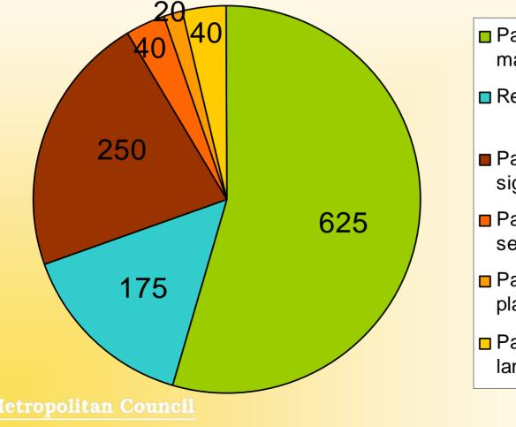
Parking lost due to mandatory elements Remaining on-street parking Parking lost due to nonsignalized ped crossings Parking lost due to secondary station access Parking lost due to 3-car platforms Parking lost due to minimize lane transitions
